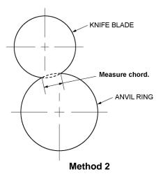
Measure the chord of the intersection between the knife blade and anvil ring.
