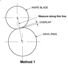
Measure blade overlap directly along the common centerline of the knife blade and anvil ring.
