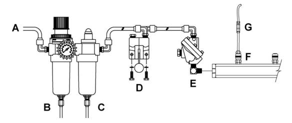
• Tidland recommends installing a 3-way slider valve **(F)** and quick disconnect **(G)** in the air supply line for each knifeholder to provide individual knifeholder actuation required for setup. All pneumatic components are available from Tidland.
