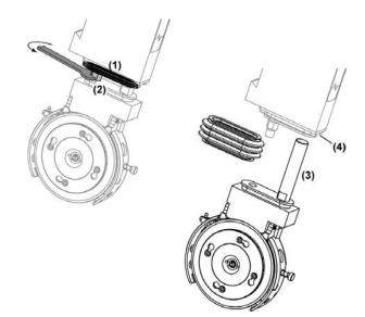
**Do not** remove the cant angle guide rod (3) from the cartridge assembly. **Do not** remove the cant angle adjustment plate (4) from the upper body.
